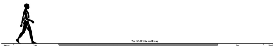
Fig. 1 Schematic representation of the GAITRite walkway setup. Subjects started 2 m in front of and ended 2 m behind the actual GAITRite walkway to ensure they would have a constant walking speed
